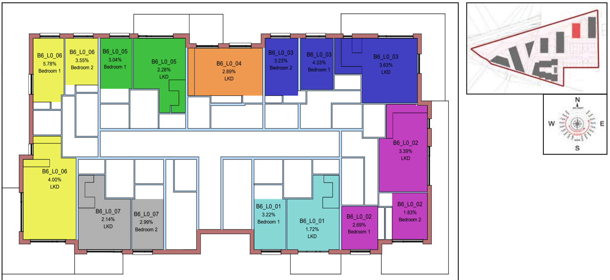
Figure 5.18: Floor plan of assessed building (L), Keyplan highlighting the assessed building (R).
